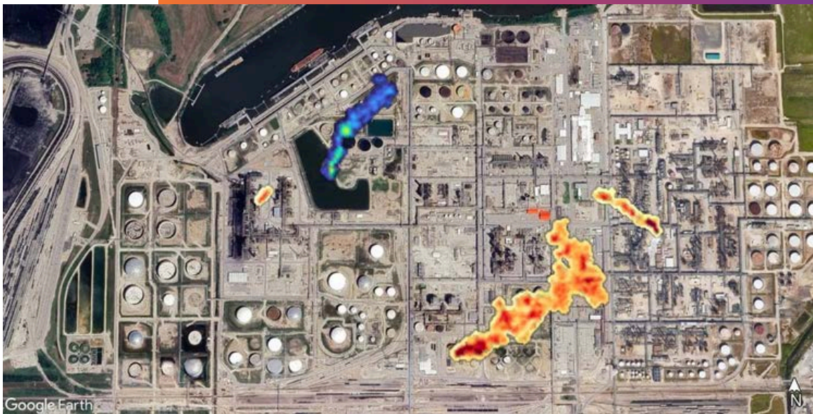
Plumes of methane and CO 2 observed by Carbon Mapper airborne surveys. Source: Carbon Mapper data portal .
